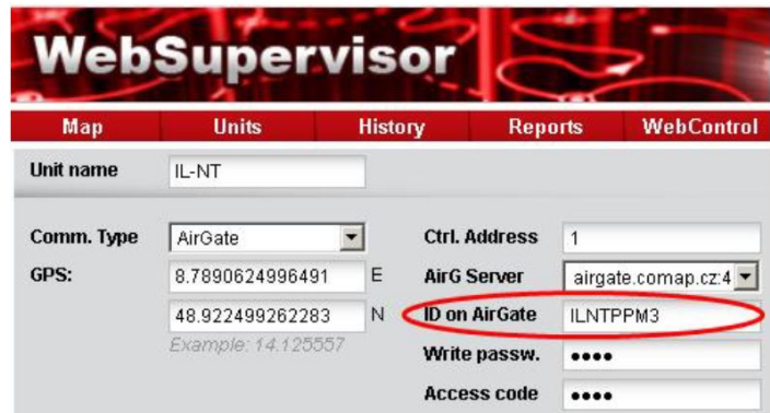
Image 9.11 WebSupervisor: AirGate Connection
